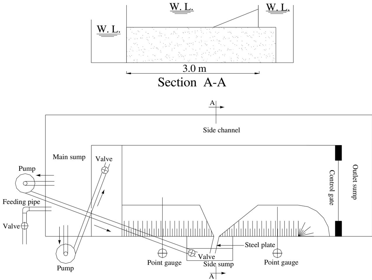
Fig.1. Longitudinal profile of the flume
