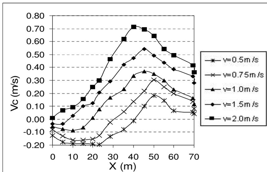
Fig.6. The measured cross current velocities at the outlet of the intruded construction, groups No. 7, 8, and 9
