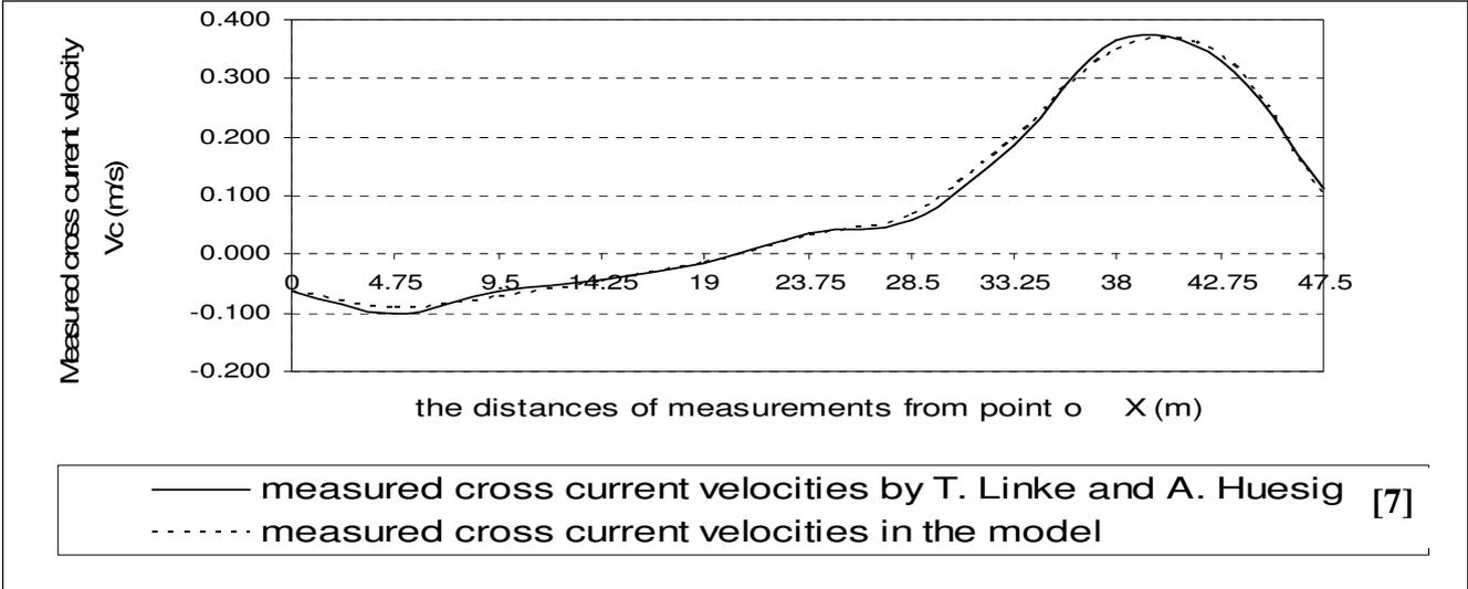
Fig.3. Comparison of measured cross current velocities at the outlet by Tobias [7], and by the author in HRI's flume
