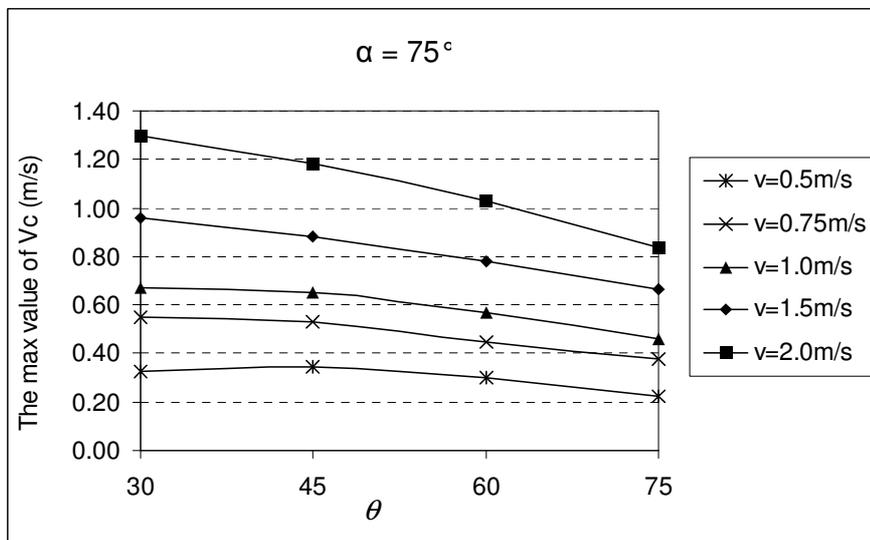
Fig.9. Variation of ( $\theta$ ) with ( $V_c$  max.) for different values of ( $V$ ) for  $\alpha = 75^\circ$
