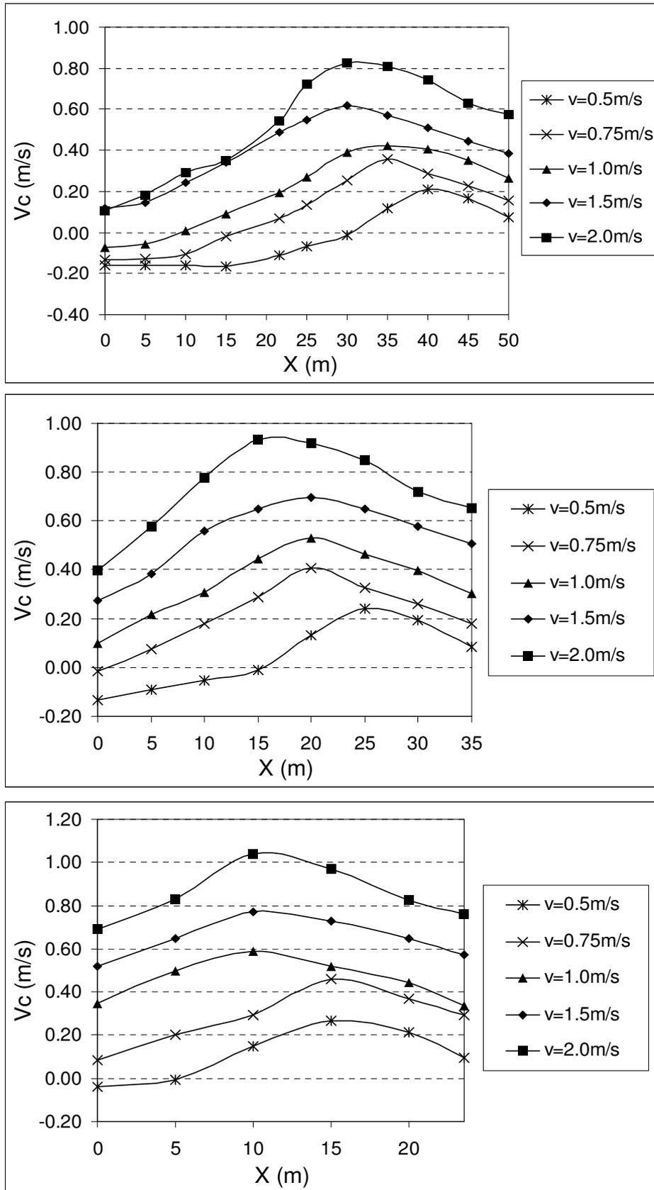
Fig.7. The measured cross current velocities at the outlet of the intruded construction, groups No. 10, 11, and 12
