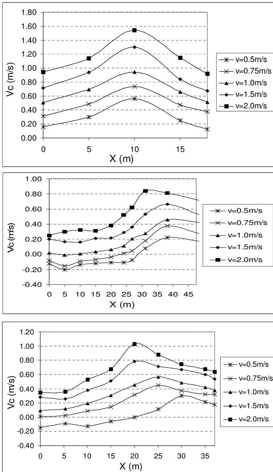
Fig.5. The measured cross current velocities at the outlet of the intruded construction, groups No. 4, 5, and 6
