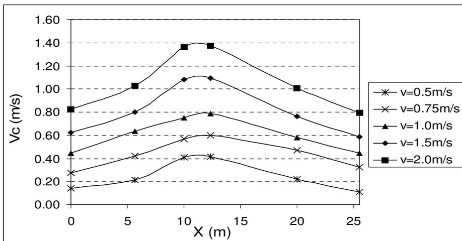
Fig.4. The measured cross current velocities at the outlet of the intruded construction, groups No. 1, 2, and 3
